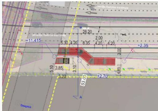
2: RAMP 2 - Proposal A - Staircase+Lift (n.60 risers H 15.10 cm)
